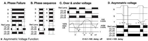
(The highest voltage of phase a,b,c,)-(The lowest voltage of phase a,b,c)
